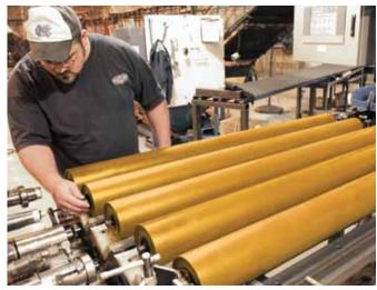
Cat ® steel rolls going through an automated five-stage assembly and testing process.
