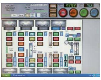
The computer panel of the roll assembly machine graphically monitors and controls the five stages of the assembly process.
