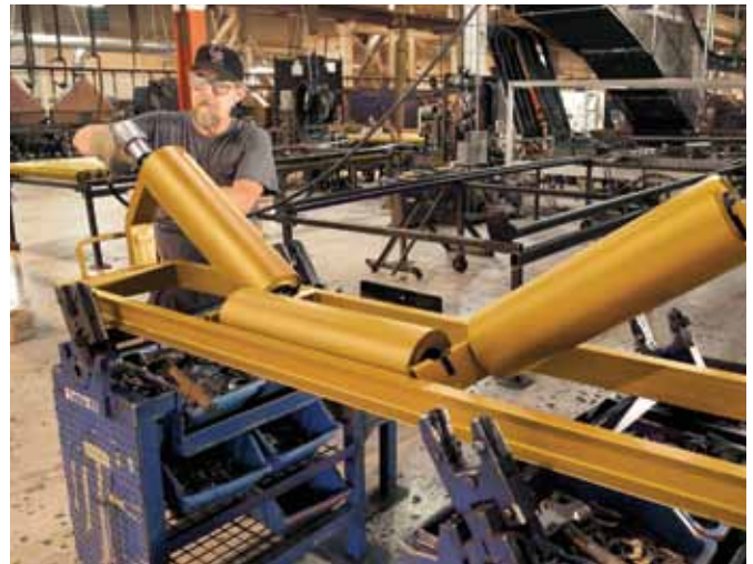
Cat® steel rolls going through an automated five-stage assembly and testing process.
