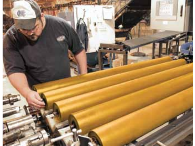
Cat® steel rolls going through an automated five-stage assembly and testing process.
