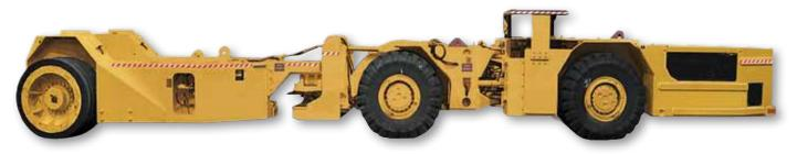
SH150 roof support trailer for CL10 and CL15 models
