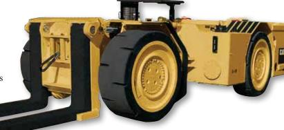
The SH640 D comes ready to operate with heavy-duty forks as standard. A range of attachments is available to turn the SH640 D into a utility vehicle between longwall moves.
