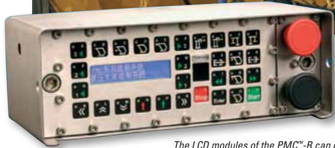
The LCD modules of the PMC™-R can display text in a wide variety of languages.
