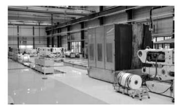
Three shearers at different stages in the manufacturing process: From the shearer on the left which is ready for equipping to the one on the right which has successfully completed all test procedures and is being prepared for shipping.
