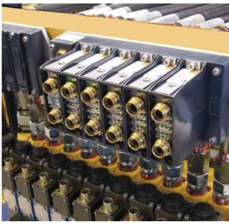
Intrinsically safe CIOS™ block with state-of-the-art Ethernet communication
