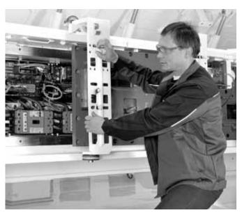
The robust mainframe protects the electrical boxes from cutting and haulage forces; door handling system for easy access to the electrical compartments.
